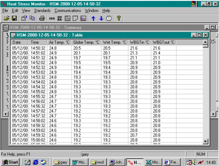
*A real time option is also selectable from a drop down tab menu, which allows monitoring of data direct via the PC.*
